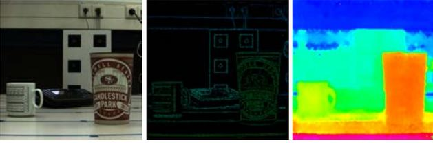
Figure 3: Recordings of a Raytrix camera. Left: Synthesized total focused image. Center: Raw depth image. Right: Filled depth image.
