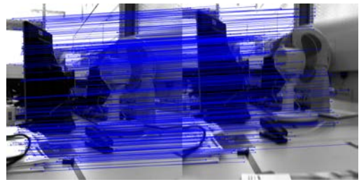
Fig. 3. Resulting matches for two consecutive images, after next neighbor search and slope filters.
